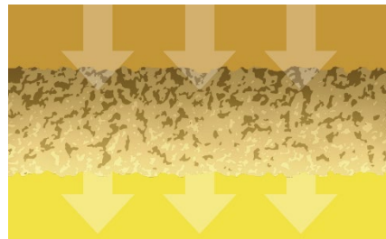
Prime Filter envelopes trap particulate AND adsorb dissolved impurities for cleaner, fresher, longer-lasting oil.
